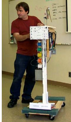
Jim Ubersetzig presented a method a method for determining position within a room using a laser emitter and sensor on the robot which rotates to look for three corner reflectors mounted on a wall. He says this method is being used by members of a couple other robot clubs since he published it a few years ago.
